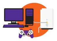
For wired devices, you can connect them directly to the **GO Smart Wi-Fi Beacons** using an **Ethernet cable** by plugging them into the **yellow LAN port**.
