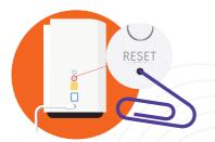
If you run into issues during setup, a **factory reset** might be required. To do this, using a **paper clip**, hold down the **RESET button** found at the **back of the Beacons**, until the front **light starts flashing red** (this will take approximately **12 seconds**).
