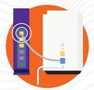
**STEP 3:** Unbox the first GO Smart Wi-Fi Beacon and use the supplied Ethernet cable to connect one end to the **blue WAN port on the Beacon**, and the other end to any of the **yellow ports 1-3** on the modem.
