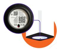
**STEP 9: Unbox your other GO Smart Wi- Fi Beacon** and before powering it on, on your mobile phone, **tap on Scan code** to utilise the QR scanner to capture the code located under your Beacon.
